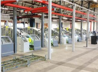
Finally, the coils are transported directly over an additionally constructed access way to the stranding machines in production. This avoids longer storage time and time loss. It also reduces costs and setup times, and optimises material flow. The new spooling centre is then optimally integrated into the supply chain.
